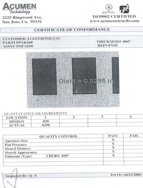
FIGURE 6. Stencil for PowerPAK SO-8
