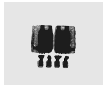
c) X-Ray of Part Placement
