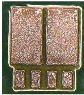
a) Solder Paste Application
